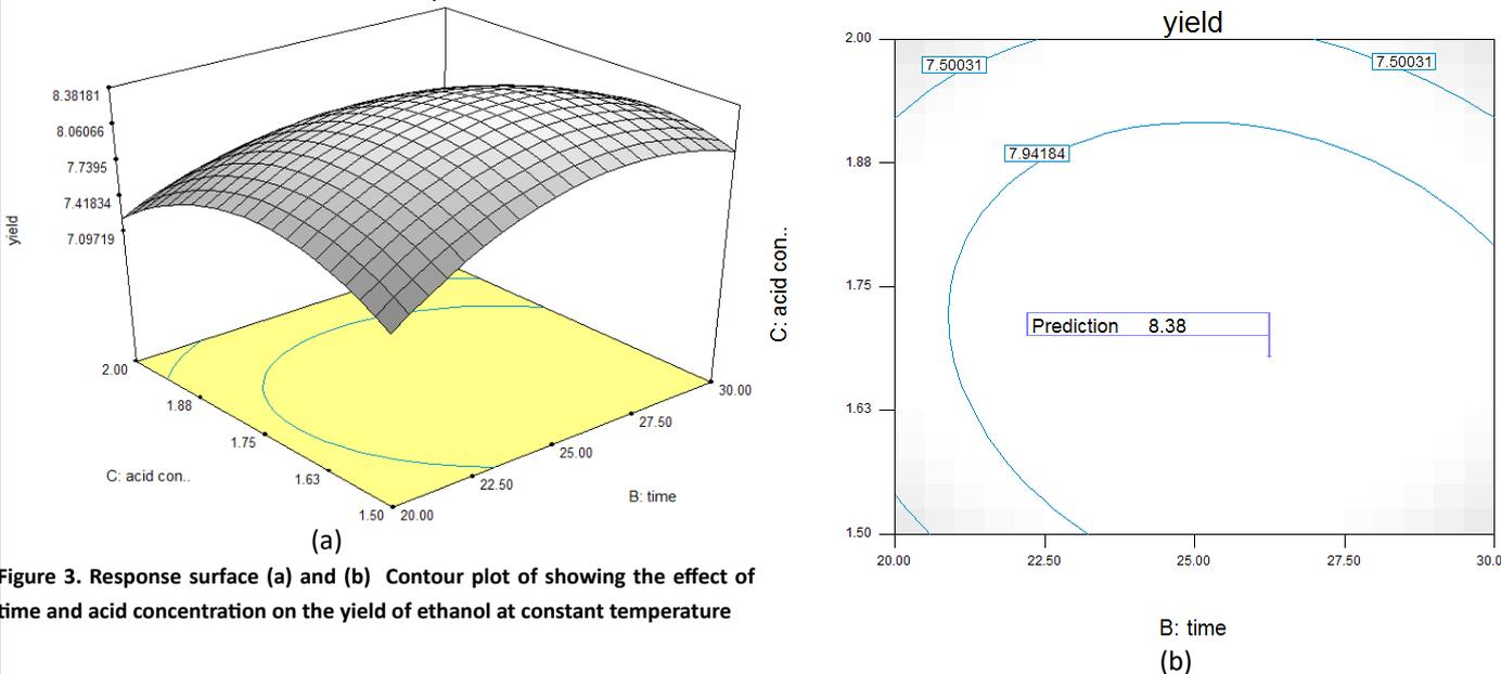
Figure 3. Response surface (a) and (b) Contour plot of showing the effect of time and acid concentration on the yield of ethanol at constant temperature
