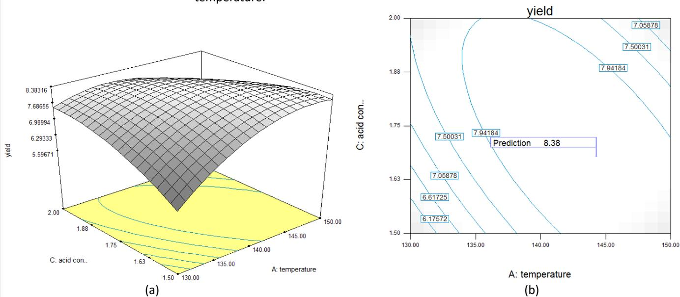
Figure 2. (a) Response surface plot and (b) Contour plot showing the effect of temperature and acid concentration at the constant time
