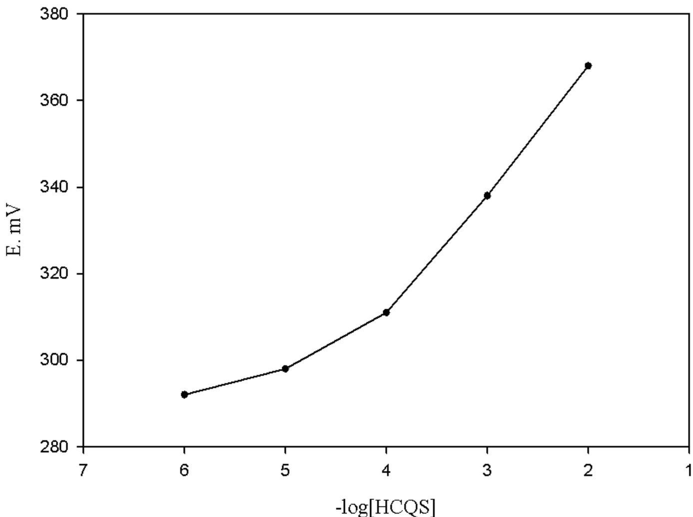
Fig. 2: Calibration curve of HCQS coated graphite sensor
