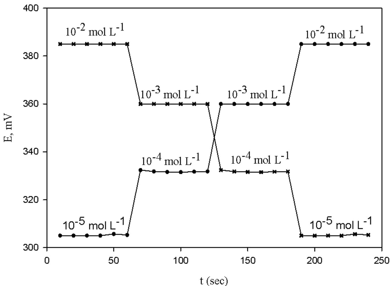
Fig. 3: The dynamic response time of CGS for step changes in concentrations of HCQS from low to high and vice versa
