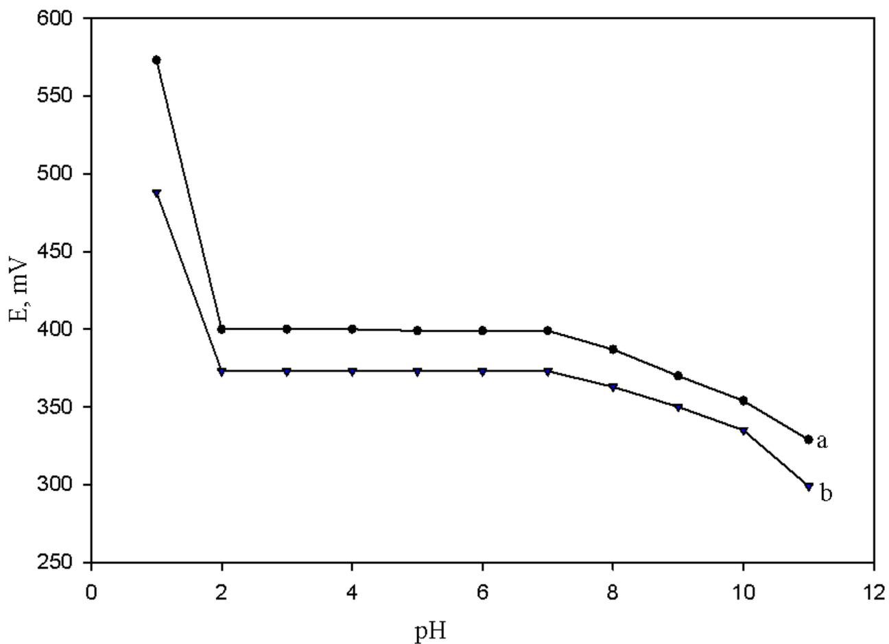
Fig.5: Effect of pH of the test solutions on the potential response of CGS a) 1.0 × 10<sup>-3</sup> and b) 1.0 × 10<sup>-4</sup> mol L<sup>-1</sup> of HCQS solution
